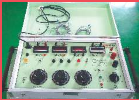
It is 100A 1 PH Relay Testing Set with Digital Meters. It is also said to be secondary injection kit used for the testing of control and relay panel
