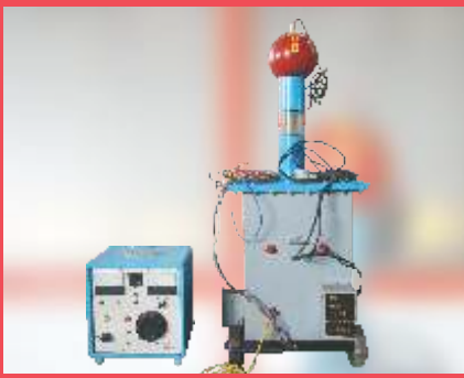
It is High voltage injection kit used for testing of all type of HT and LT panel
