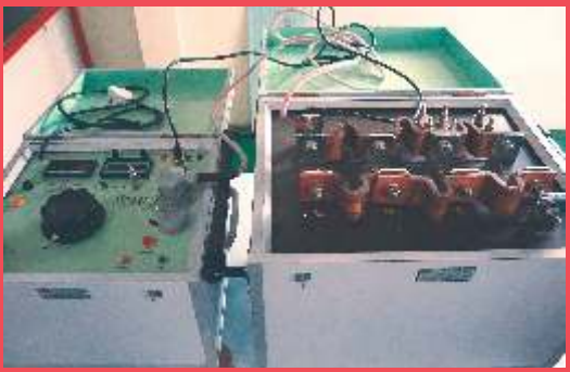
It is Primary injection kit Testing Set With Digital Meters. Having two parts of control unit and loading unit
